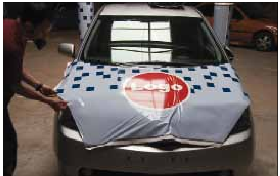
Glass is a term that refers to the state of the film when it has no wrinkles. Wrinkles on the film mean that bubbles will result if it's squeegeed.
