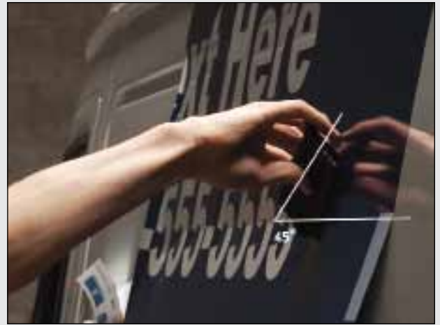
The 45-degree angle allows for the largest area to be applied while giving the air underneath the film time to escape.
