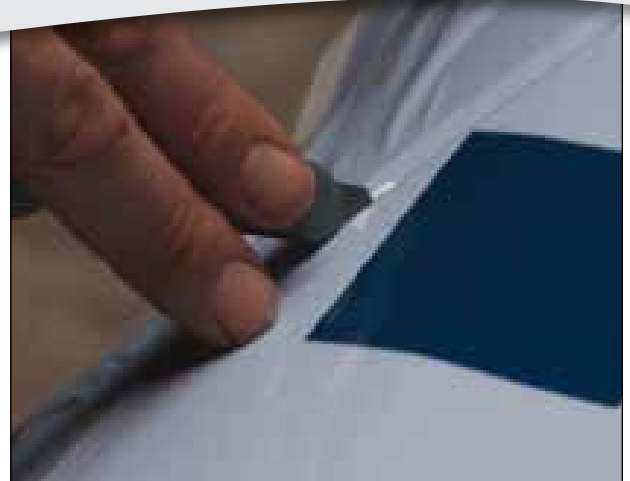
Have a knife that holds the blade securely and let the blade do the cutting. For me, I think the NT Cutter A-551P knife is ideal for vehicle installations.
