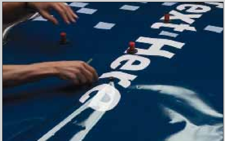
Relief cuts are made on the film to reduce tension, which allows it to lay flat on the vehicle. Relief cuts can be made on corners and on raised objects like door handles or antennae.
